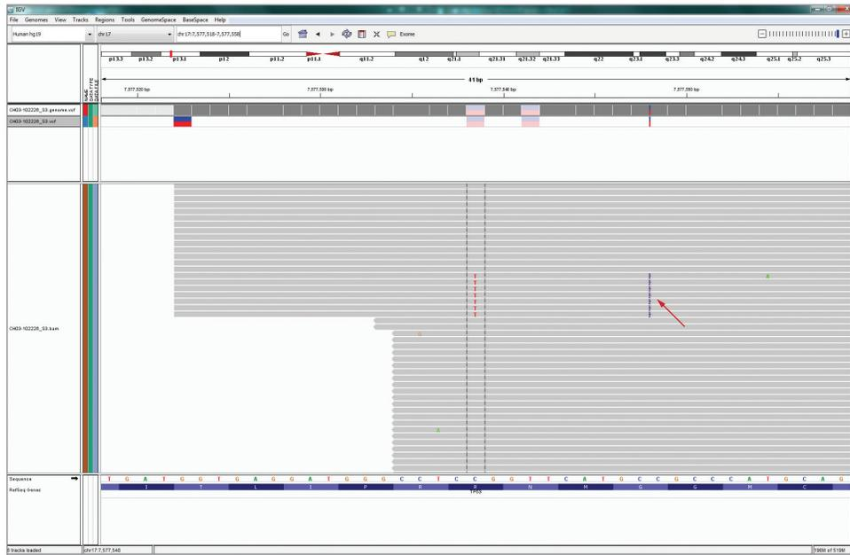
**Figure 2:** Integrated Genome Viewer (IGV) screenshot of a TP53 mutation from the Seraseq Solid Tumor Mutation Mix. The six-base Internal Quality Marker (IQM) insert is highlighted.
