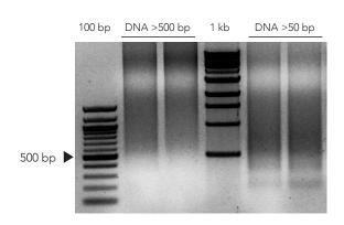
Equivalent amounts of DNA resolved in a 1% agarose/TAE/EtBr gel show binding conditions may be adjusted with the  $\textit{Quick}\text{-DNA}^{\text{\tiny{M}}}$  FFPE Kit to selectively isolate DNA >50 bp or >500 bp. 100 bp and 1 kb DNA ladder shown.
