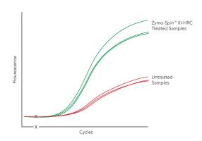
Quick-RNA<sup>™</sup> Environmental Kits removed PCR inhibitors using the Zymo-Spin<sup>™</sup> III-HRC Filter. RNA was isolated from a *Nicotiana sp.* leaf, spiked with humic acid, with and without the Zymo-Spin<sup>™</sup> III-HRC Filter. RT-qPCR detected early amplification for the filter treated samples compared to the untreated samples ( $c_p = 30$  vs. 31).
