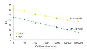
HeLa cells were titrated down to a single cell, and DNA and total RNA were extracted using the Quick-DNA/RNA $^{\text{\tiny{M}}}$  Microprep Plus Kit. Analysis by RT-qPCR shows high linear recovery of DNA & RNA down to the single-cell level (n=2).
