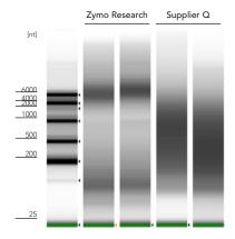
RNA isolated with the <code>Quick-RNA</code> FFPE Kit is higher quality (left) compared to a Supplier Q kit (right). Quality assessed using the Agilent 2200 TapeStation $^{\circ}$  system.
