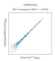
RNA purified from TRIzol® using Direct-zol™ RNA compared to an unbiased method (mirVana $^{\text{\tiny{TM}}}$ , Ambion). Data is highly correlated (2837 overlapped miRNA:  $r^2 = 0.9706$ ). Analysis was performed using miRNA-Seq (MiSeq®, Illumina).
