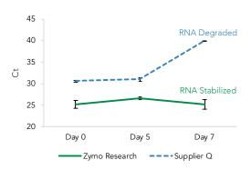
RT-qPCR shows the Zymo Research workflow stabilizes RNA, while the Supplier Q workflow leads to degradation. Whole blood was stored up to 7 days at ambient temperatures and extracted at the indicated time points using the Zymo Research or Supplier Q preservatives and workflows.
