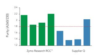
RNA was cleaned-up using the RCC $^{\text{\tiny{M}}}$  kit and a Supplier Q kit (n=4). RNA purity (measured by A260/230) was greater than 1.8 for the RCC $^{\text{\tiny{M}}}$  kit but not for the Supplier Q kit.
