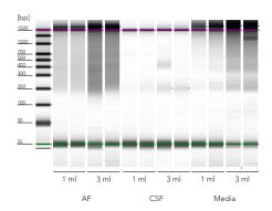
Amniotic fluid (AF), cerebrospinal fluid (CSF), or spent HeLa cell culture media (Media) were used to isolate cell-free nucleic acids using Quick-cfDNA/cfRNA $^{\infty}$  Serum & Plasma Kit. Endogenous cell-free DNA from each sample type was visualized using the Agilent 2200 Tapestation $^{\odot}$  system.
