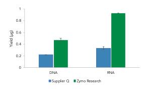
DNA and total RNA recovery is higher using the Quick-DNA/RNA $^{\text{TM}}$  Microprep Plus Kit compared to a Supplier Q kit. Nucleic acids were extracted from 50K HeLa cells (n=2).
