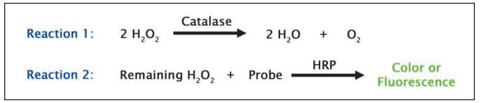
Assay Principle for the OxiSelect™ Catalase Acitivity Assays. Catalase present in samples converts hydrogen peroxide into water and oxygen (Reaction 1). Any remaining hydrogen peroxide that is not converted reacts with a colorimetric or fluorometric probe in the presence of horseradish peroxidase (Reaction 2) to produce a color or fluorescence which is measured in a plate reader.
