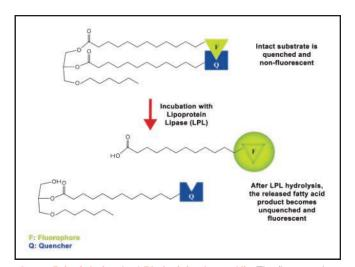
Assay Principle for the LPL Activity Assay Kit. The fluorogenic substrate is initially quenched and non-fluorescent. Upon cleavage of the probe by incubation with lipoprotein lipase (LPL), fluorescence can be measured at an excitation of 342 nm and emission of 400 nm.
