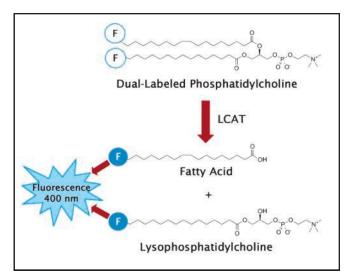
Assay Principle for the LCAT Activity Assay Kit. The close proximity of fluorescence labels on a dual-labeled fluorogenic probe keeps the fluorescence quenched. Upon cleavage of the probe by LCAT, fluorescence of the monomers can be measured at an excitation of 342 nm and emission of 400 nm.
