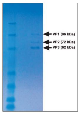
Electrophoretic Profile of Purified AAV2-GFP.
