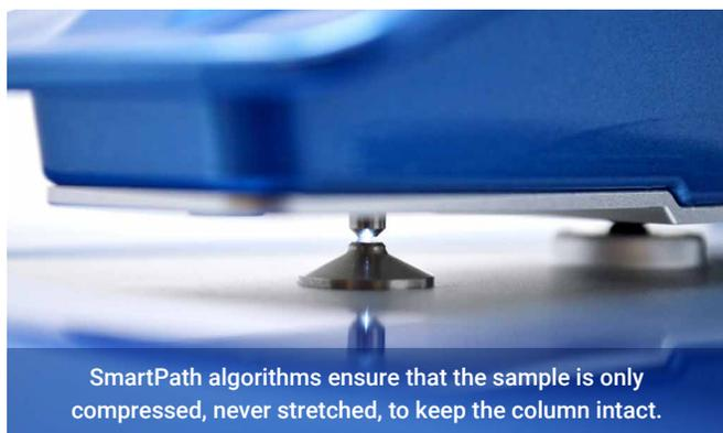
SmartPath algorithms ensure that the sample is only compressed, never stretched, to keep the column intact.
