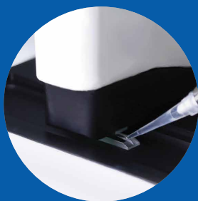
Load Cell Suspension into Sample Chamber
