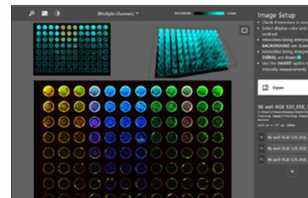
Arrays and plate-based assays can utilize the Array module's grid-based analysis system which includes options for normalization and presence/absence detection.
