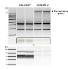
(Top) High quality broad size-range DNA-free RNA is purified from human epithelial cells using the Direct-zol<sup>M</sup> procedure compared to a preparation from Supplier Q (1% agarose/TAE gel).
