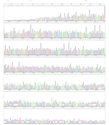
Sequencing chromatogram of plasmid DNA pGEM<sup>®</sup> purified using the **Zyppy™ Plasmid Miniprep Kit**. The DNA was labeled with ABI BigDye v3.1 terminators, cleaned using the **ZR DNA Sequencing Clean-up Kit™ (D4050, D4051)** and sequenced on an ABI 3730x/ DNA analyzer.
